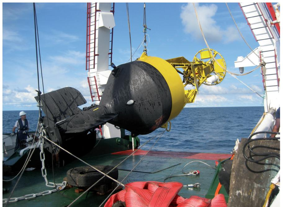
in the concept of tsunami warnings. Since a few years concepts have been developed to use GPS technology for the monitoring of the instantaneous sea level. This concept was introduced into GITEWS to increase the system reliability for tsunami warnings. Using a modern GPS receiver and additional sensors, the newly developed buoys are able to independently measure the sea level to an accuracy of better than 5 cm under a wide range of sea state conditions.
