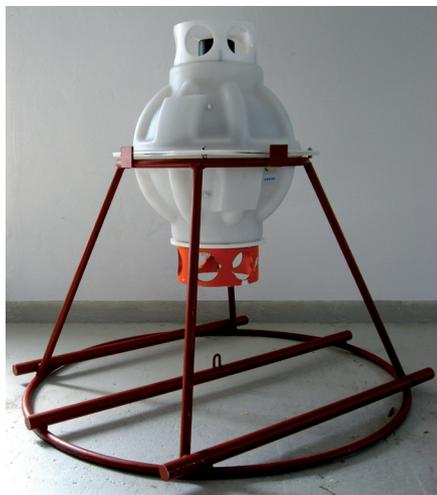
nologies of the new millennium, PACT integrates the entire sea-floor package (pressure gauge, data logger and analyzer, acoustic modem, acoustic release and relocation aids) into a single unit, i.e. a standard benthos sphere. PACT, thereby, reduces costs, maximizes reliability and minimizes the deployment efforts while maximizing reliability and maintenance intervals.
